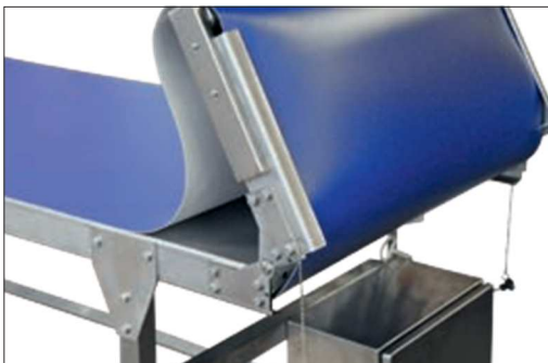
NIRO confectionery conveyor belt with folding device and scraper knife
